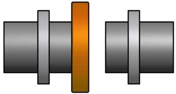
**Figure 6.2.1.4 Insert Facing tool between pipe ends**
