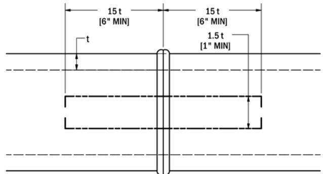
**Figure 7.1 Sample Strip dimensions (ASTM D 2657)**
