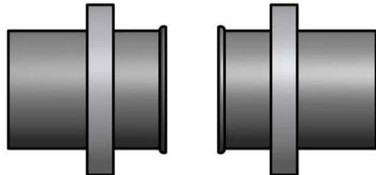
**Figure 6.2.2.4 Remove heater and inspect fusion surfaces.**
