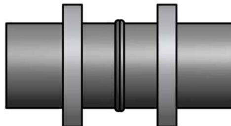
**Figure 6.2.2.3 Bring ends together with fusion force.**
