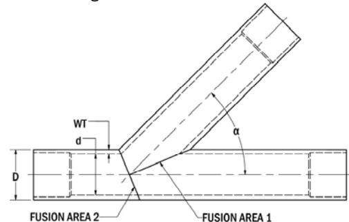
Figure 4.1 Dimensions used in Fusion Area Calculations
