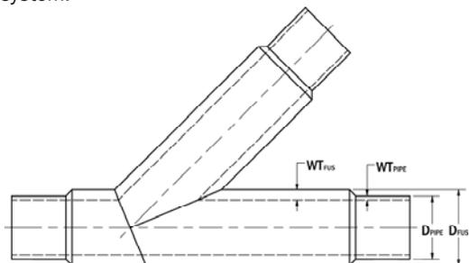
Figure 3.1 Dimensional Overview of IDC Y-Lateral
