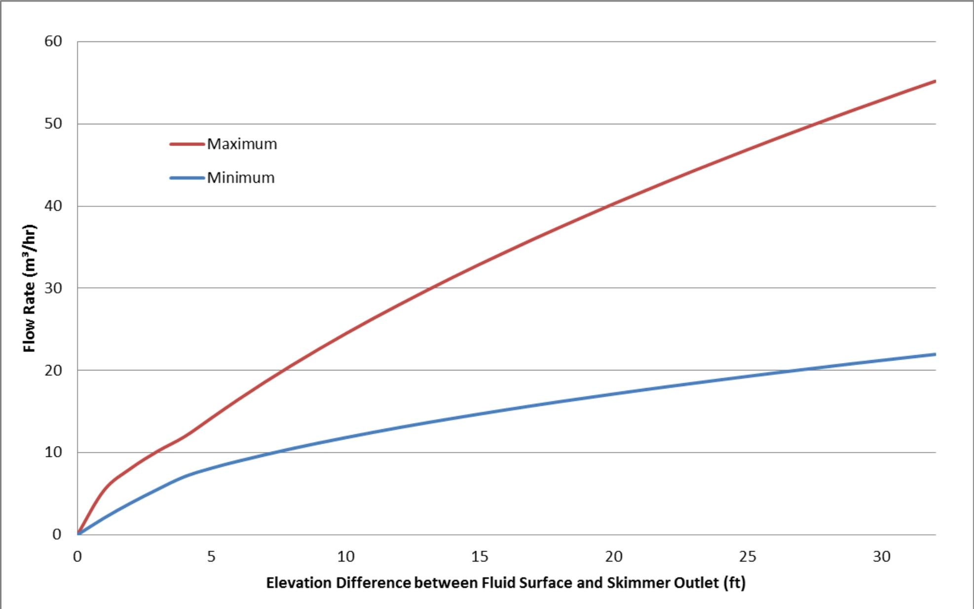
Figure 1: Extrapolated skimmer flow rate for medium-heavy crude oil at room temperature.
