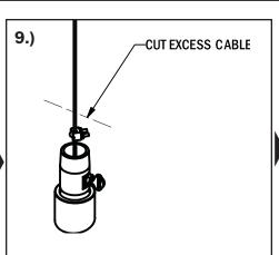
Cut off the excess cable, leaving enough to grab onto if future adjustement is required.
