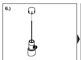
Remove the housing cap from the float guide assembly and pull out the cable clamp and excess cable.
