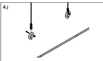
Attach the strap forks to the corresponding rings of the float cable guide anchor with the 10-32 UNF machine screws and lock nuts provided. Ensure that the guide cables are not twisted.
