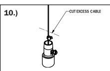
Cut off the excess cable, leaving enough to grab onto if future adjustement is required.
