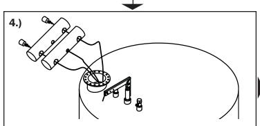
Run the guide cables through the two guide holes of the poly float and attach the float cable from the gauge head.
