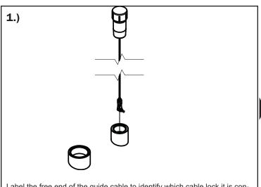
Label the free end of the guide cable to identify which cable lock it is connected to. Insert the end of the cable with the strap fork from the float guide cable lock assembly into the 1-1/4 NPT couplings and feed down into the tank.
