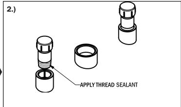
Apply thread sealant on the bottom threads of the float guide cable lock assembly housing and install into the 1-1/4 NPT coupling with the pipe wrench. Repeat with the second float guide cable lock assembly.
