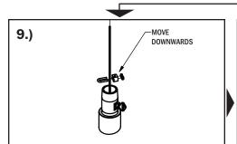
Loosen the cable clamp using the 5/16 wrench, and reposition as near to the cable lock pocket as possible.
