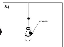
Turn thumb screw clockwise to secure cable. Use the 9/16 wrench to tighten the sealing nut.
