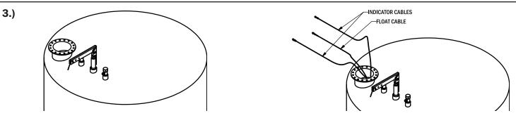
Using the hook, reach into the tank through the thief hatch and grab the float guide cables, the float cable from the gauge head and pull them out of the thief hatch.
