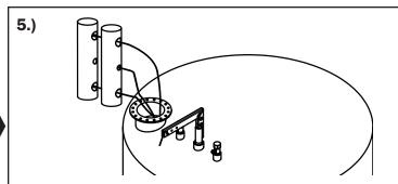
Feed the cables back into the tank from the hatch, followed by the float. Hold the guide cable between the float and the anchor, and ease the anchor into the tank through the thief hatch and onto the tank floor.
