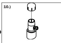
Position the remaining cable and cable clamp into the pocket and replace the housing cap with the pipe wrench. Repeat 5-9 with second float gude cable lock assmbly.
