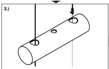
From inside the tank, run each cable through corresponding guide hole on the float.
