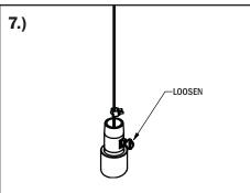
Turn the thumb screw counter clockwise to loosen cable. Pull the cable and cable clamp upwards until taut.
