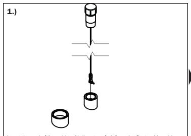
Insert the end of the cable with the strap fork from the float guide cable lock assembly into the 1-1/4 NPT couplings and feed it down into the tank.
