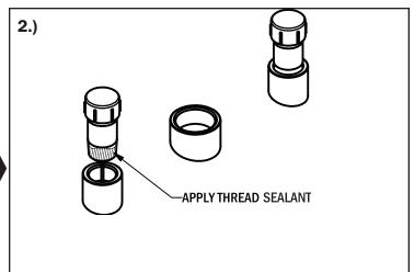
Apply thread sealant on the bottom threads of the float guide cable lock assembly housing and install into the 1-1/4 NPT coupling with the pipe wrench. Repeat with the second float guide cable lock assembly.
