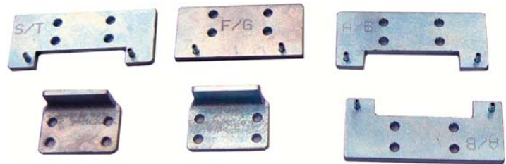
Below: Modular RACI Vice Tool jaw sets (l - r) for S&T, F&G and A&B sizes.
