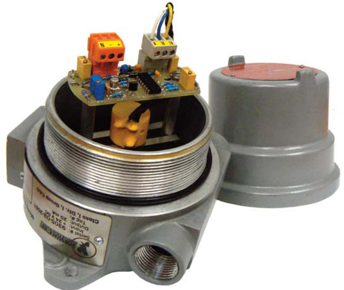
Above: Goshawk Transmitter with cover removed
